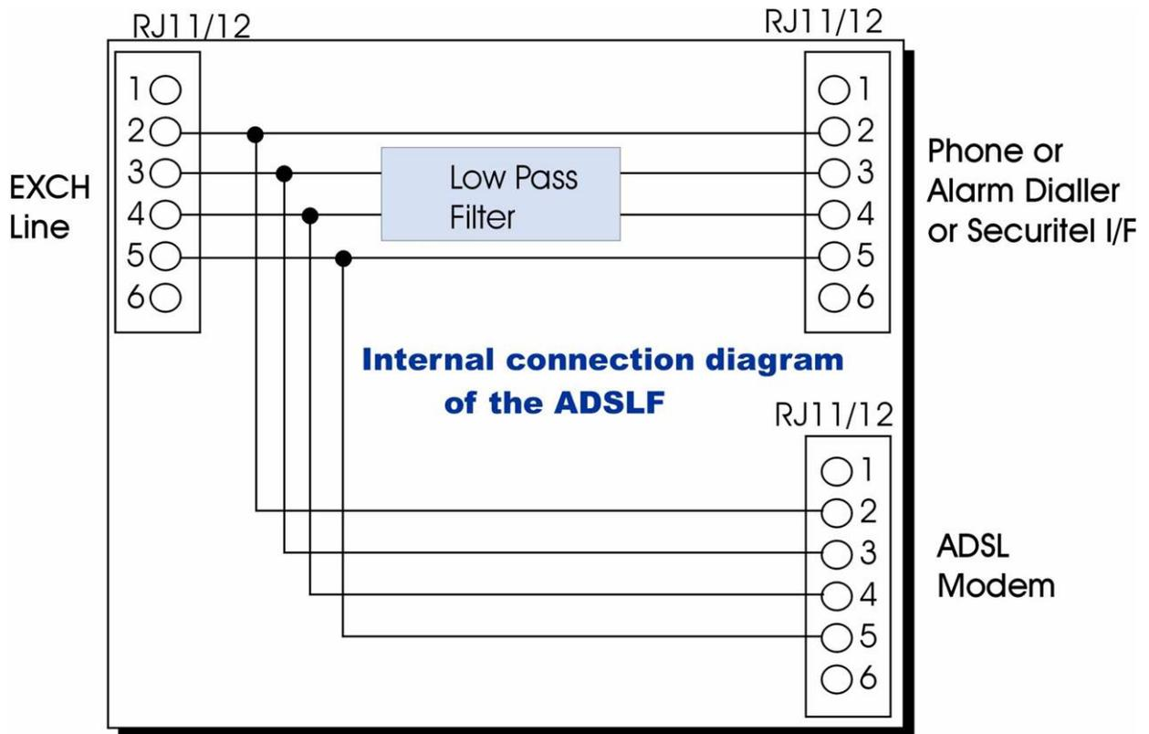
***MCMs ADSLF filter splitter - internal connections***
